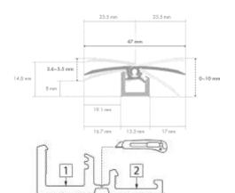
The **aluminium** profile consists of two parts, which you can separate along the break line. Hold the profile firmly in both hands and start by prying one side up and down. Do this step by step over the entire length of the profile until both parts have completely separated.
