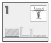
Fix the rail to the underfloor with screws. Screw them into the pre-drilled holes in the rail. Use 3x30 mm screws.
