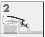
Now place the bottom part of the aluminium profile in the rail. When you do this, the wing of the moulding sits on the higher side of the rail.
